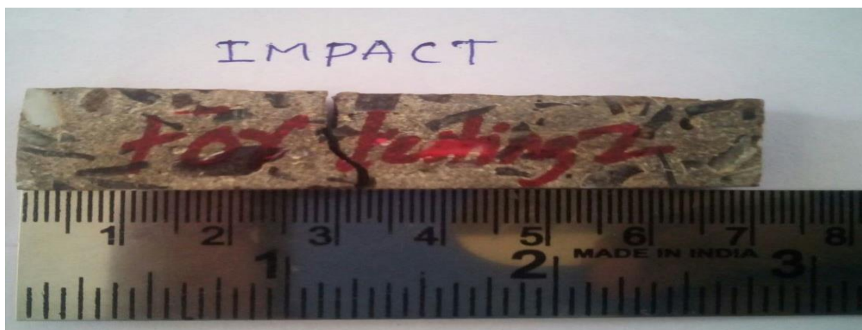
Fig. 4 Cracked DRFP composite specimen under impact test.
