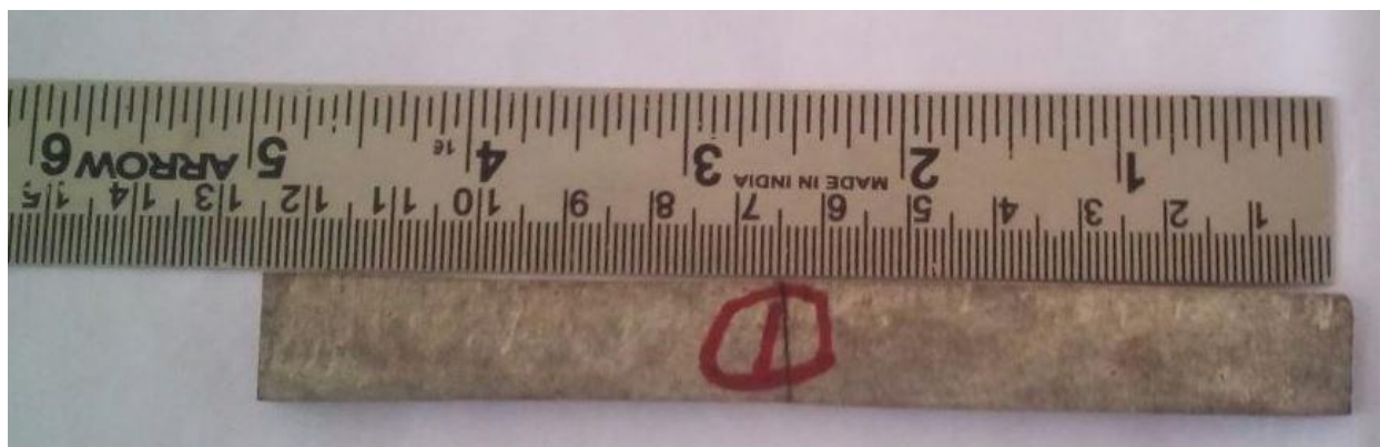
Fig. 3 Cracked DRF composite specimen under flexural strength test.
