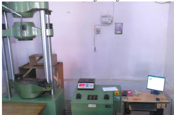
Fig. 3.5 UTM setup for Elongation Test
