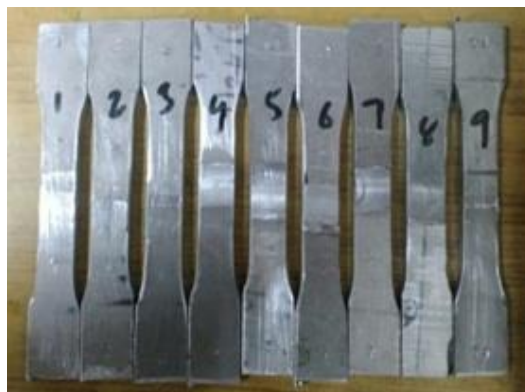
Fig. 3.7 Tensile test specimen before failure
