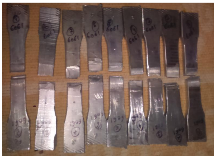
Fig. 3.8 Tensile test specimen after failure
