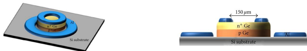
Figure 5: Design of the Ge-based light emitting diode. (a) Isometric schematic of the device structure showing the Ge mesa on top of a p-type Si substrate with Al ring contacts. (b) Cross-section schematic of the device structure. Figures are taken from [68].
