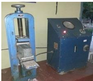
Concrete specimens testing for flexural strength
