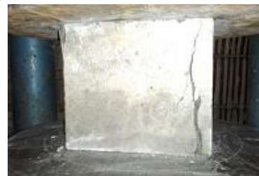
Concrete cube specimens testing for compressive strength
