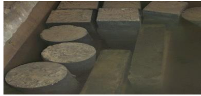
Curing of concrete specimens
