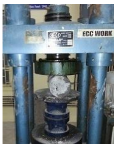
Concrete specimens testing for split tensile strength
